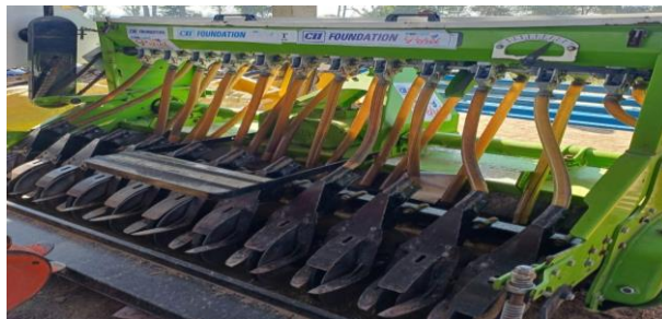
Super Seeder (Mix stubble in soil, prepare land & sow)
