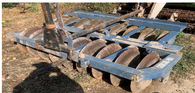
Harrow (Breaks up & smoothen soil bed)
