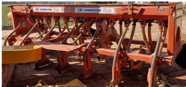
Happy Seeder (Manages residue through incorporation)
